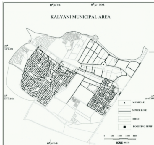
Fig. 11: Underground sewerage line Source: Kalyani Municipality, 2010
