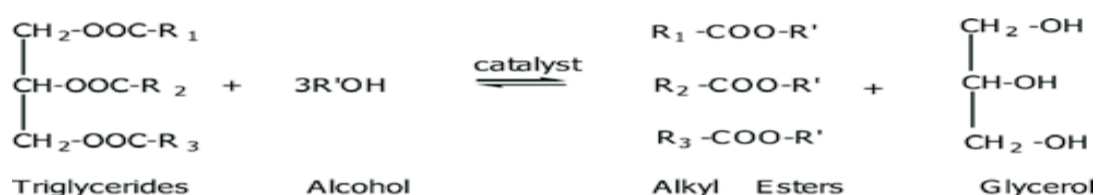
Fig. 1 Transesterification of triglyceride with alkyl alcohol
