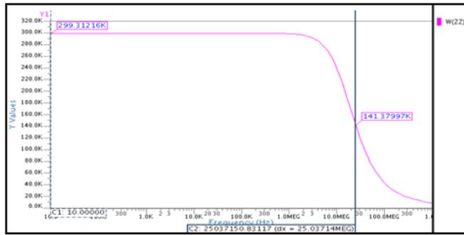
Figure 4.20: Impedance at Z terminal for 0.18µm CMOS technology
