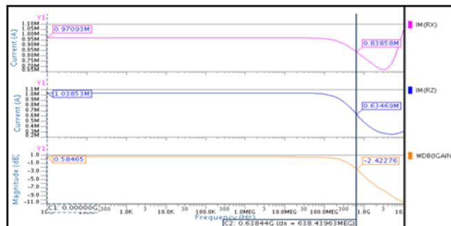
Figure 4.12: Gain and Bandwidth for 0.25µm CMOS technology
