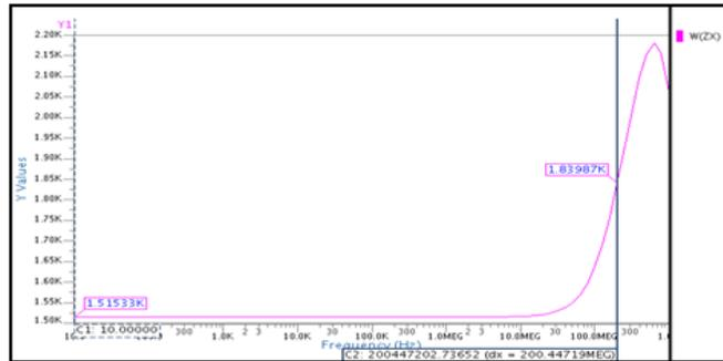
Figure 4.3: Impedance at X node for 0.05 $\mu\text{m}$  CMOS technology
