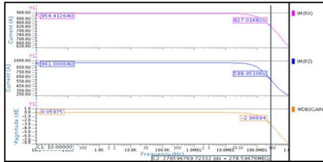
Figure 4.17: Gain and Bandwidth for 0.18µm CMOS technology
