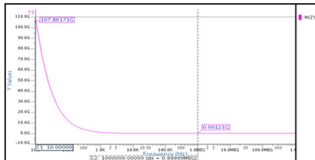
Figure 4.19: Impedance at Y terminal for 0.18µm CMOS technology
