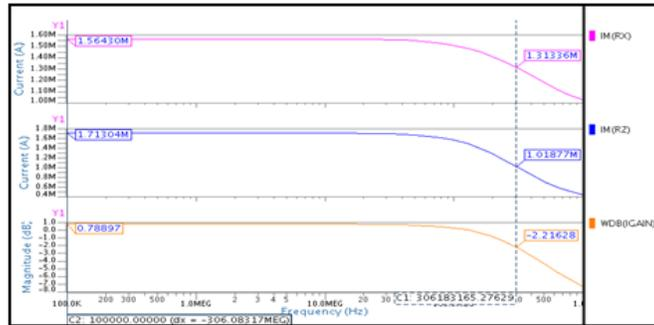
Figure 4.2: Gain and Bandwidth for 0.05 $\mu\text{m}$  CMOS technology
