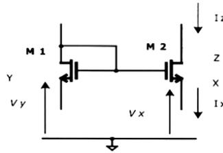
Figure 3.3: CCII characteristics in nMOS current mirror
