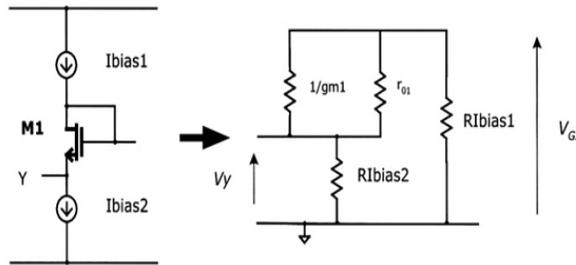
Figure 3.4: Half nMOS current mirror and its small signal equivalence
