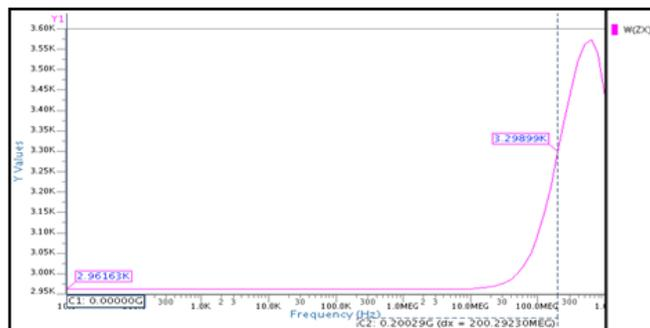
Figure 4.18: Impedance at X terminal for 0.18µm CMOS technology
