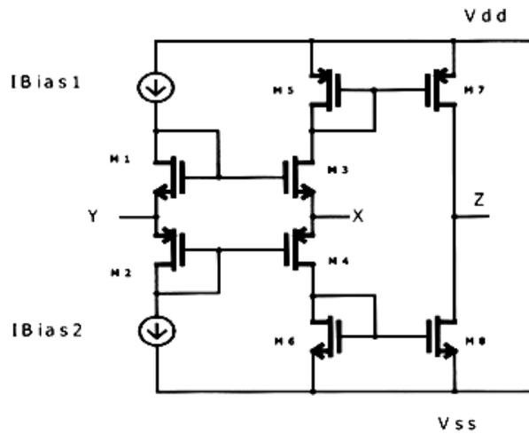
Figure 3.6: Class AB CCII based on Current Mirrors
