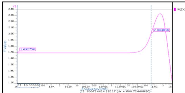
Figure 4.8: Impedance at X terminal for 0.35µm CMOS technology
