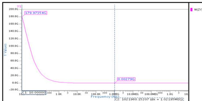
Figure 4.9: Impedance at Y terminal for 0.35µm CMOS technology
