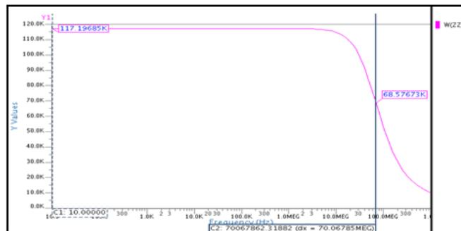
Figure 4.15: Impedance at Z terminal for 0.25µm CMOS technology
