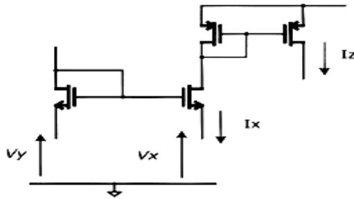
Figure 3.5: Current Mirrors used for Positive CCII
