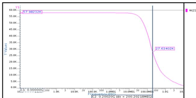
Figure 4.10: Impedance at Z terminal for 0.35µm CMOS technology
