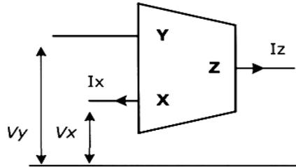
Fig 1.1 Block representation of Current Conveyor II
