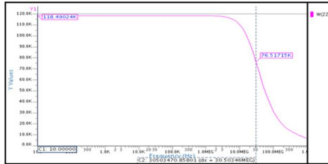
Figure 4.5: Impedance at Z node for 0.05μm CMOS technology
