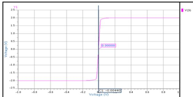
Figure 4.6: Offset for 0.05μm CMOS technology
