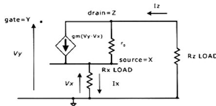
Figure 3.2: Small Signal Circuit for nMOS
