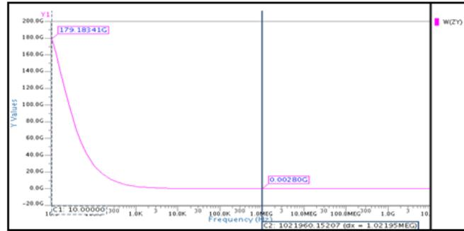
Figure 4.14: Impedance at Y terminal for 0.25µm CMOS technology
