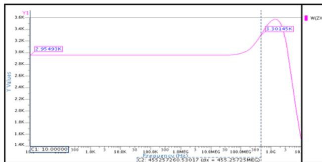
Figure 4.13: Impedance at X terminal for 0.25µm CMOS technology
