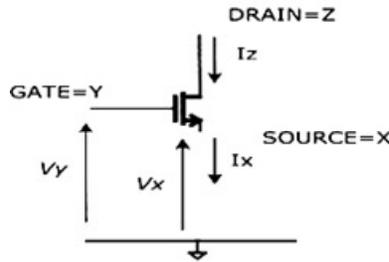
Figure 3.1 nMOS transistor and its equivalence with CCII
