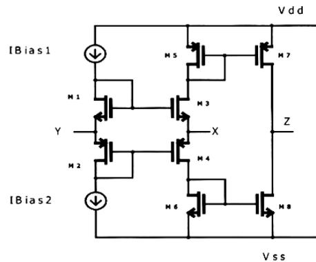
Figure 4.1: CCII Based on Current Mirrors
