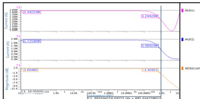
Figure 4.7: Gain and Bandwidth for 0.35μm CMOS technology
