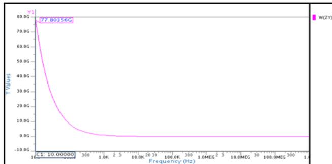
Figure 4.4: Impedance at Y node for 0.05μm CMOS technology
