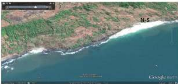
Plate 5: Google image exhibiting N30°W and N-S mega joints as well as beach deposits controlled by them. Location: near Adivre village
