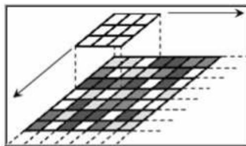
**Fig. 7: Generation of a new image by filtering operation; selected window moves both row-wise and column-wise and calculates new values.**
