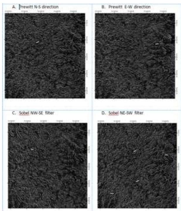
Fig.8: Subset images generated by Sobel and Prewitt filters, Arrows: enhanced lineaments
