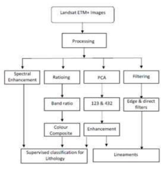
**Fig. 2: Flowchart for digital image processing methods used.**
