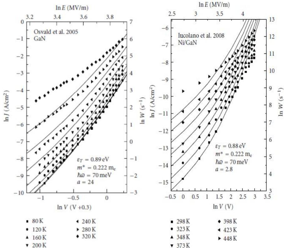
**Fig.2: Comparison of I-V dependences for metal/n-GaN Schottky diode from Figure 2 [5] (symbols) with theoretical  $W(E,T)$  against  $E$  dependences (solid curves), computed using parameters:  $\epsilon T = 0.89$  eV,  $m^* = 0.222 m_e$ ,  $\hbar \omega = 70$  meV,  $a = 2.4$ .**
