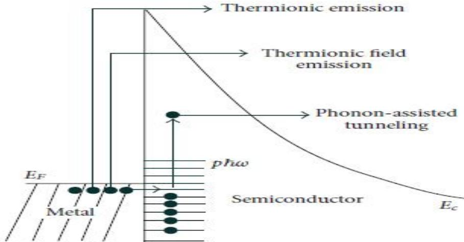
**Fig 1.Engery level diagram of the metal/ Semiconductor contact**
