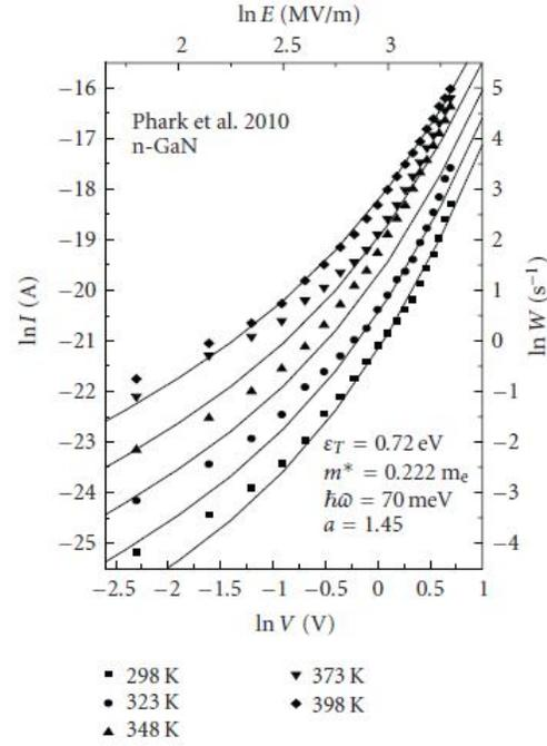
**Figure 4:** The  $I$ - $V$  characteristics of Au/ $n$ -GaNano-Schottky diode represented from Figure 2 [19] (symbols) fitted to theoretical  $W(E,T)$  against  $E$  dependences (solid curves). Parameters for computation:  $\epsilon T = 0.5$  eV,  $m^* = 0.222m_e$ ,  $\hbar\omega = 40$  meV,  $a = 2.0$ .
