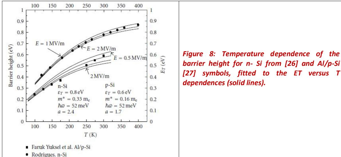
**Figure 8: Temperature dependence of the barrier height for n-Si from [26] and Al/p-Si [27] symbols, fitted to the ET versus T dependences (solid lines).**
