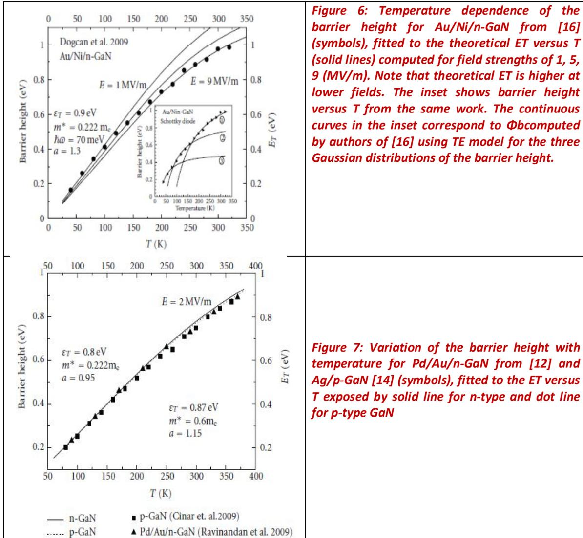
**Figure 6:** Temperature dependence of the barrier height for Au/Ni/n-GaN from [16] (symbols), fitted to the theoretical ET versus T (solid lines) computed for field strengths of 1, 5, 9 (MV/m). Note that theoretical ET is higher at lower fields. The inset shows barrier height versus T from the same work. The continuous curves in the inset correspond to  $\Phi_b$  computed by authors of [16] using TE model for the three Gaussian distributions of the barrier height.
