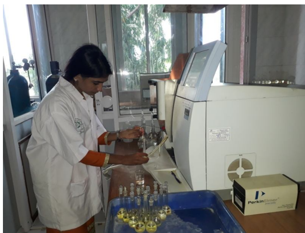
Fig.1-Nutrient analysis by Atomic Absorbance spectrophotometer
