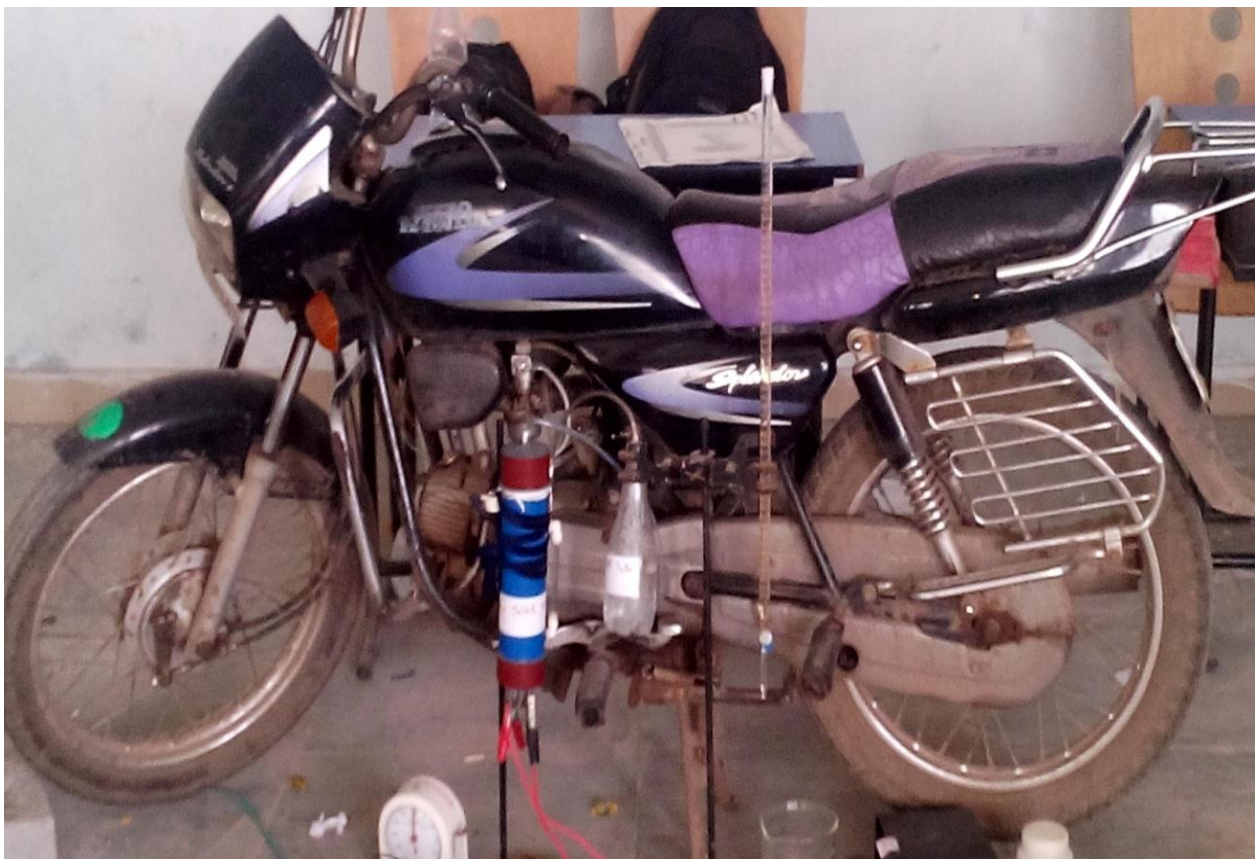
Fig5.2: Single cylinder four stroke spark ignition engine setup.
