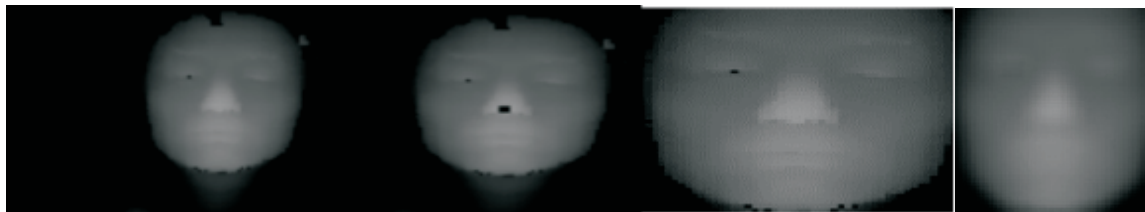
Fig.2. (a) Depth image (b) nose finding (c) sliced image (d) After removing the noise and the filling of holes.
