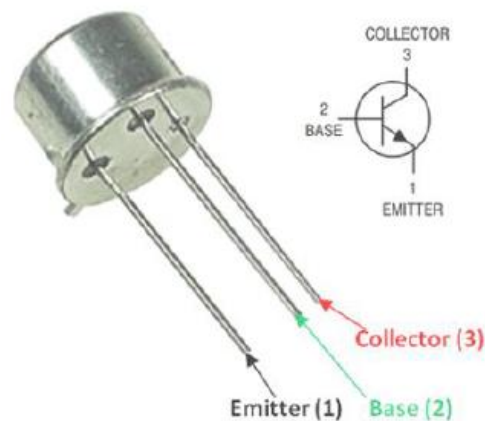
Figure 1. The official design of the commercialized 2N2219-NPN transistor by STMicroelectronics Inc. features the schematic electronic symbol. Adapted from [25].
